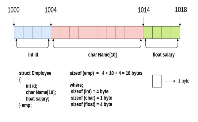
Here, struct is the keyword; employee is the name of the structure; id, name, and salary are the members or fields of the structure. Let's understand it by the diagram given below:
