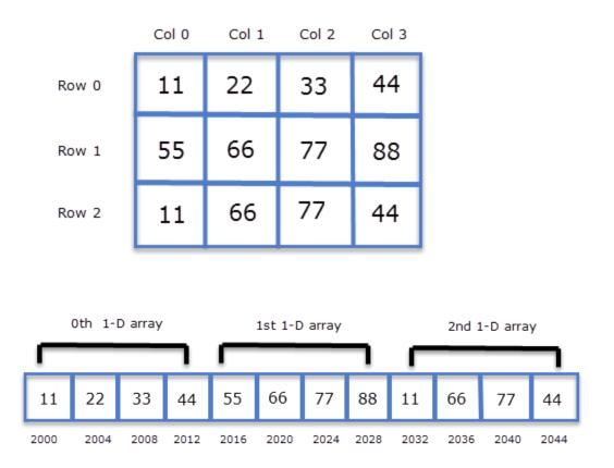
Note:- name of a 1-D array is a constant pointer to the 0th element. In the case, of a 2-D array, 0th element is a 1-D array. Hence in the above example, the type or base type of arr is a pointer to an array of 4 integers. Since pointer arithmetic is performed relative to the base size of the pointer. In the case of arr, if arr points to address 2000 then arr + 1 points to address 2016 (i.e 2000 + 4\*4).
